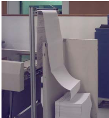
Inserter infeed non-powered feeding an inserter from a Lasermax Roll Systems MiniRack.
